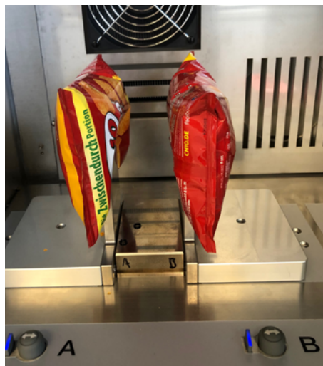
Specialized cartridge enables simpler testing of pouch samples.
