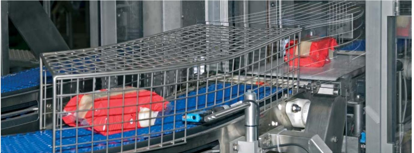
If the package passes the CO<sub>2</sub> test, it is returned to the production line and a new package is loaded into the test chamber. If, on the other hand, the package is leaking, it is pushed into a reject box. All the processes are fully automatic.
