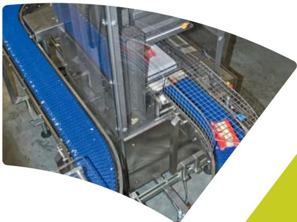
*Packages are tested on a parallel conveyor containing Dansensor LeakMatic.*
