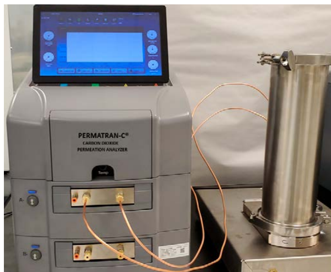
Figure 4. MOCON PERMATRAN-C 4/30 used to test pre-filled carbonated drink bottle
