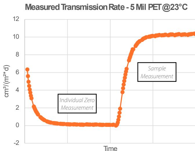
Example of Individual Zero run at the beginning of a test.
