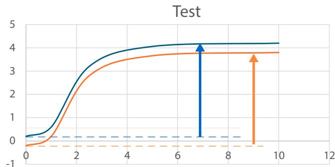
In very tight systems with low Re-Zero values, sometimes a negative value may be recorded for the Individual Zero. This is not necessarily an error but reflects changes during the test duration. The compensation still functions to provide the most accurate test result for that sample and test on that day.
