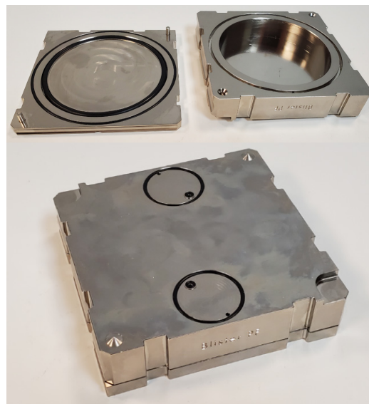
Figure 1. Blister Test Cartridge for Pre-filled Blister's WVTR testing (P/N 054-575)
