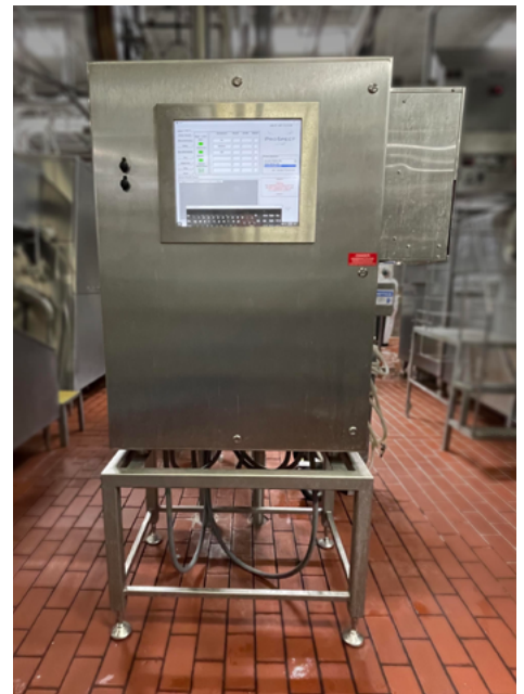
ProSpect In-line Process NIR for measurement of Fat, Moisture, Salt and SNF in butter
