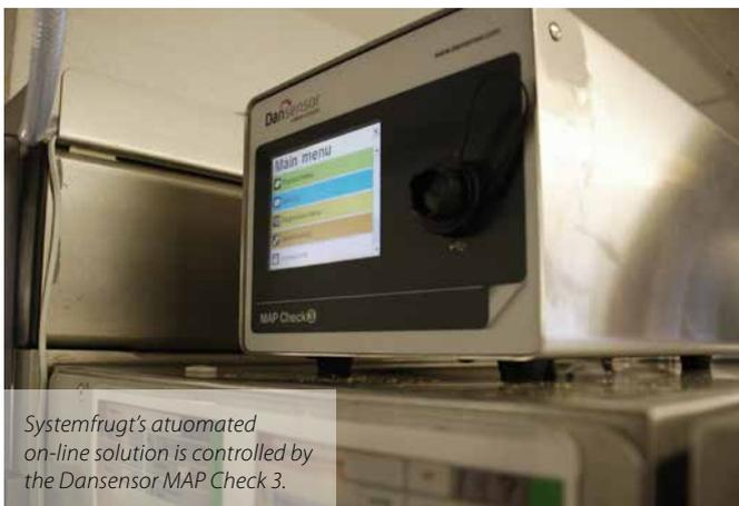
Systemfrugt’s automated on-line solution is controlled by the Dansensor MAP Check 3.
