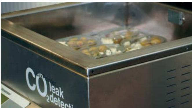
The Dansensor LeakPointer will fast and easily discover seal integrity problems on MAP packages with a minimum of 10% CO<sub>2</sub> in the gas mix.
