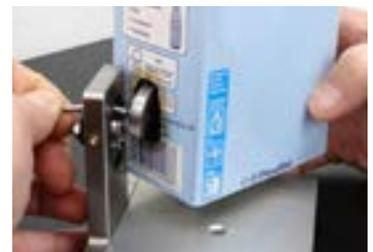
Figure 3. Place the carton sample inside a permeation analyzer
