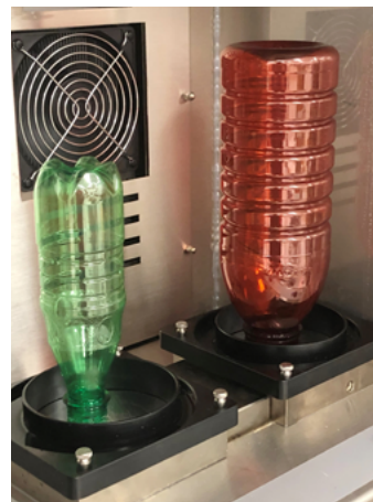
(Fig. 6) High temperature high humidity bottle testing
