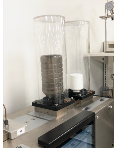
(Fig. 11) High humidity OTR bottle testing
