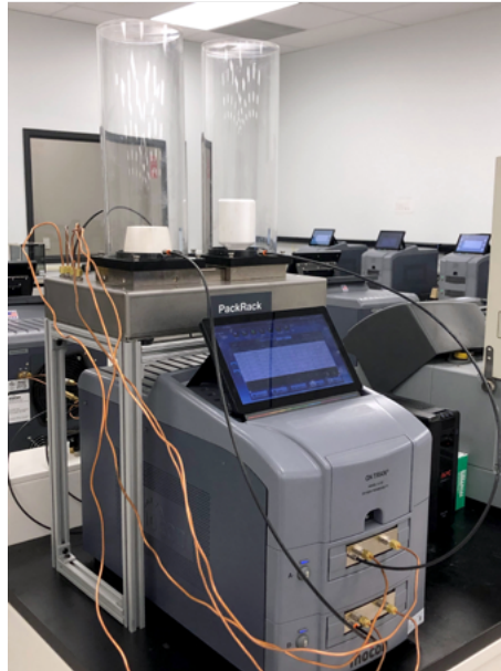
(Fig. 10) High barrier OTR testing with PackRack
