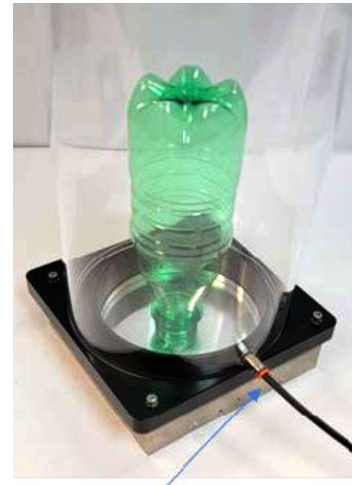
(Fig. 5B) Quick connection & gas line for test gas
