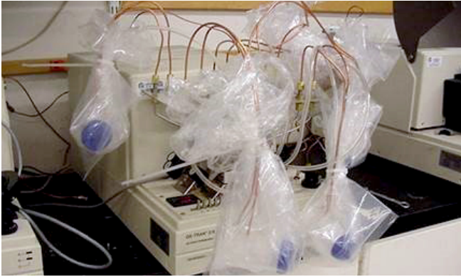
(Fig. 3) Historical testing using bags to create test gas environment.
