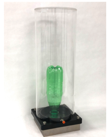
(Fig. 4D) 100% RH bottle testing setup
