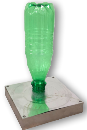
(Fig. 4B) Bottle epoxied on thin plate
