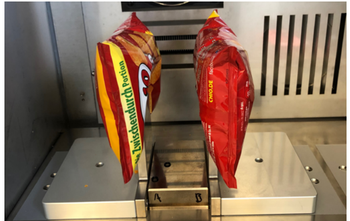
Specialized cartridge enables simpler testing of pouch samples.
