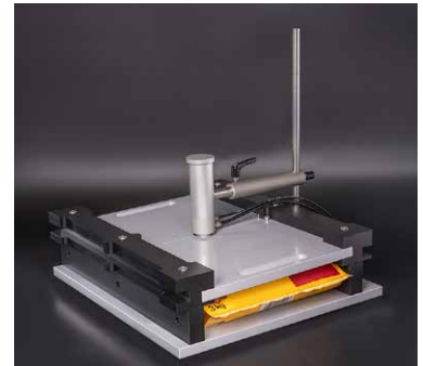
Fixture for ASTM F2054 restraining – restrains the package to ensure the pressure affects the package sealings in the correct way
