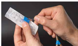
A septum ensures an airtight seal and protects the package from tearing. Different types of septa are suited to different packages and needles.
