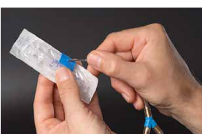
A septum ensures an airtight seal and protects the package from tearing. Different types of septa are suited to different packages and needles.
