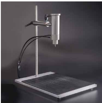
Basic stand – the test head can be combined with a sharp or blunt needle or a tube adaptor
